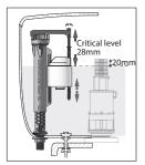
Set JOLLYFILL inlet valve to water line (the water line should be marked on the inside wall of your cistern). To do this you must lift and turn at the same time, the telescopic valve. The top of the floating cup must be at the level of the water line.
